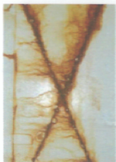
Cross cut test of epoxy paint & salt spray after 120 hours without STEEL GUARD COAT
